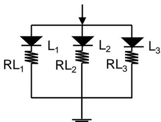
Fig.1. Recommended Circuit in Parallel Mode :
